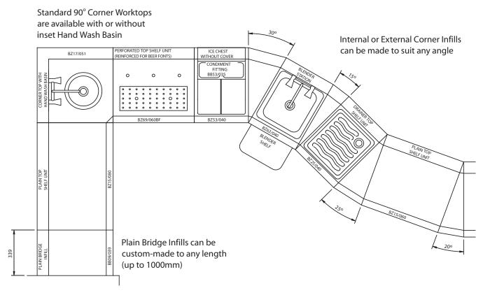
Even curved and angled bars present no problems. Standard corner worktops and custom-made infills allow a continuous bar of virtually any shape to be easily installed.
