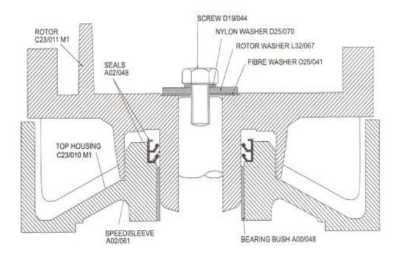
Fig 10: Seal Assembly 1204X / 1604X
