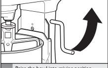
Raise the bowl into mixing position by rotating the bowl lift lever counterclockwise to the straight up position. The bowl must always be in the raised position when mixing.
