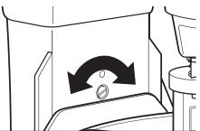
Turn beater height adjustment screw (A) slightly counterclockwise (left) to raise the flat beater; or turn clockwise (right) to lower the flat beater. Adjust so that the flat beater just clears the surface of the bowl. If you over adjust the screw, the bowl lift lever may not lock in place.
