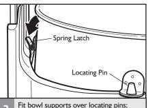
Fit bowl supports over locating pins; press down on back of the bowl until bowl pin snaps into the spring latch. If not securely snapped into place, bowl will be unstable and wobble during use.
