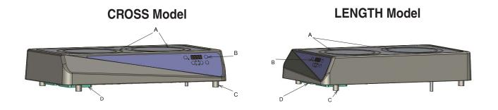
A: Hot plate - B: Control panel - C: Feet - D: Filter
