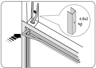
11. Position an anti-condensation cable (R8) on the front panel and fix the cable covering with 8 screws 4.2x13.
