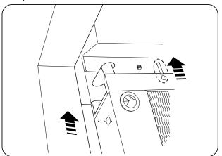
17. Fix the evaporator to the cabinet body, inserting the 4 M8x100 screws from the top.
