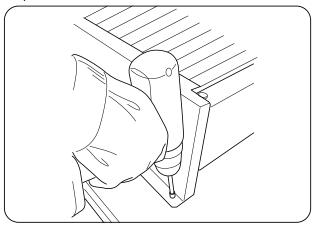
19. Take the casing with fans and insert it on the evaporating unit hinges.
