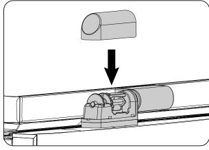
26. Adjust the latch (on the left side of the appliance) for proper support of the door seal.
