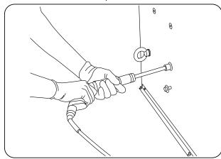
18. Fix the condensate tray to the lower inside back of the evaporator.
