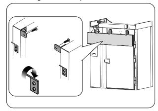
47. Fit the rear brackets with four 4.8x13 large head screws.
