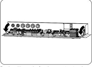
39. Run the cables, coming from the compartment, on the hole arranged in electrical system box. Close the hole with a sealant, making sure to cover any gaps.
