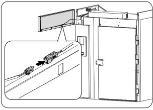
46. Hook the neutral front panel to the support brackets and fix it to the right and left side panels with screws M4.2x13.
