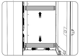
29. Fix the fan cables to the side of the evaporator with the clamps supplied. Run the cables of the two probes (compartment probe and evaporator probe, located respectively on the grille of the first fan at the top, and the other in the upper zone of the finned pack, through the hole arranged in the top.
