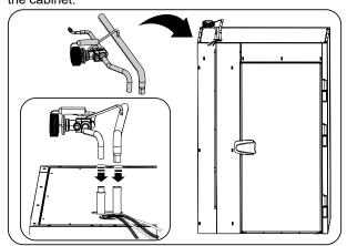
34. Position the unit delivery and return pipes on the evaporator outlet pipes and weld them (before welding the pipes, it is advisable to wrap the thermostatic valve with a damp cloth). Cover the pipes and thermostatic valve with anti condensation tube and seal the top outlet pipes with sealant, covering any join grooves.
