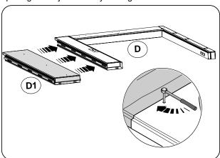
7. Join the front panel with door opening with the back and sides.
