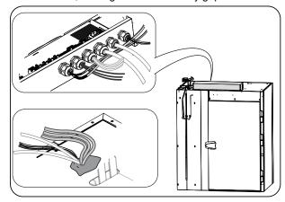
40. Connect all the cables, including those from the compartment, to the terminal block, carefully following the numbering given on them and the wiring diagrams.
