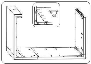
6. Take the front panel D1 and the front panel with door opening D and join them by closing the catches.
