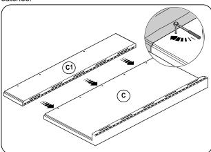
Take the back, position the left side and close the couplings. A CLICK must be heard! Do not use excessive force in closing operations.
