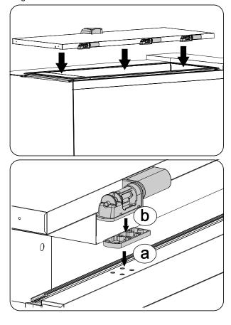
24. Fix the hinges to the cabinet with M6x35 screws.
