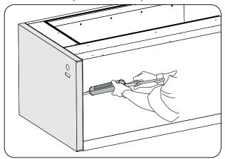
Run the heating cables (R1/2) along the cabinet trim, making them come out the hole provided on the front panel.
