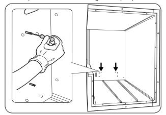
14. Take the evaporating unit, remove the side deflectors and the casing comprising the fans; position the evaporator in the cabinet body.
