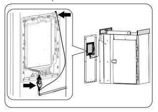
44. Hook the control panel to the support brackets.
