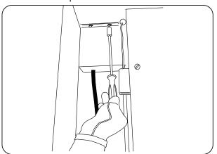
31. Fix the core probe support on the front panel near the air deflector with 2 M5x12 screws.
