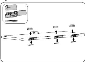
23. Place the door against the cabinet after positioning the hinge shims.
