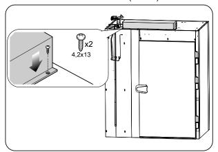
42. Fit the right and left side panels, fixing them with the appropriate screws (M4.2x13).
