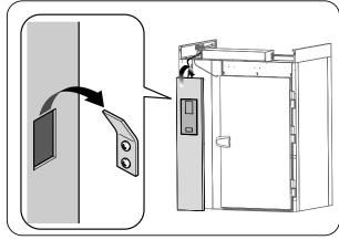
45. Connect the door micro switch wire to the neutral front panel.
