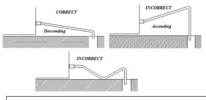
IT IS MANDATORY TO GROUND THE EQUIPMENT To avoid possible discharges on individuals or damages to the equipment, the machine should be grounded pursuant local and/or national regulations as the case may be. THE MANUFACTURER SHALL BE HELD HARMLESS IN CASE OF DAMAGES ARISING DUE TO THE LACK OF THE GROUND INSTALLATION.
