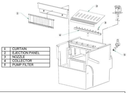
**CAUTION:** IT IS VERY IMPORTANT WHEN REPLACING THE CONTAINER THAT THE NOZZLES ARE PERPENDICULAR, AS IF TWISTED, THE EXTERNAL CUBES COULD RUN OUT OF WATER.
