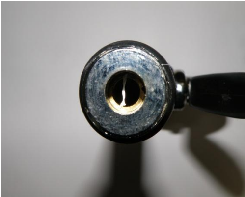
Barrel that connects to hose is flat
