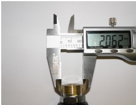
Thread diameter is approx. 20.6mm
