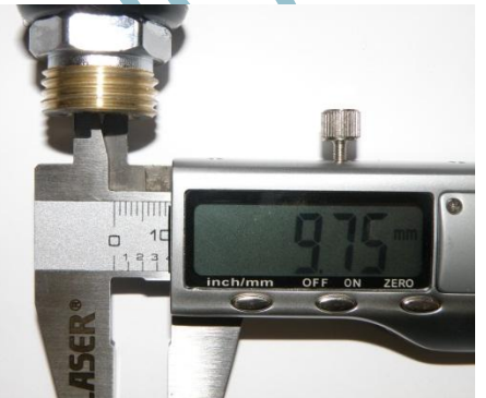
Internal barrel diameter is approx. 9.75mm
