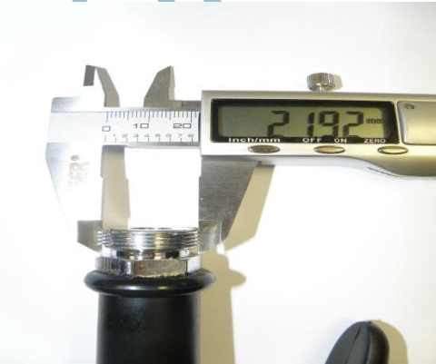
Thread diameter is approx 21.9mm
