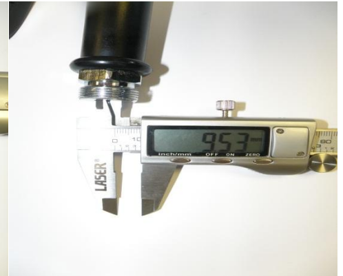
Internal barrel diameter is approx. 9.53mm
