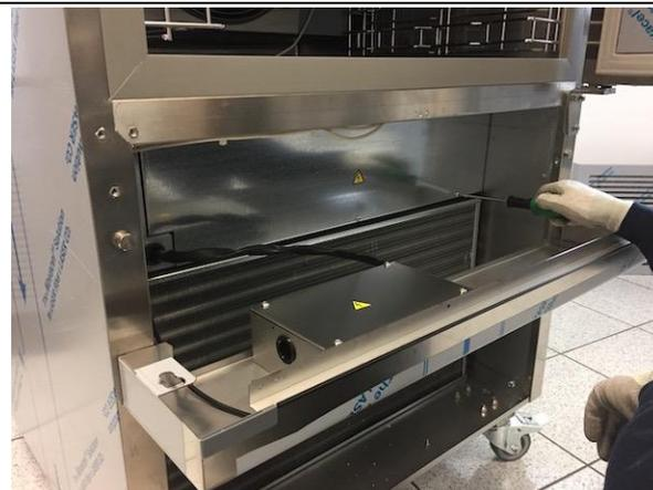
11. Cut the clamps that secure the frame resistance.
