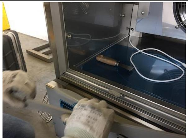
5. Loosen the two knurled knobs located on the ends of the front lower side.
