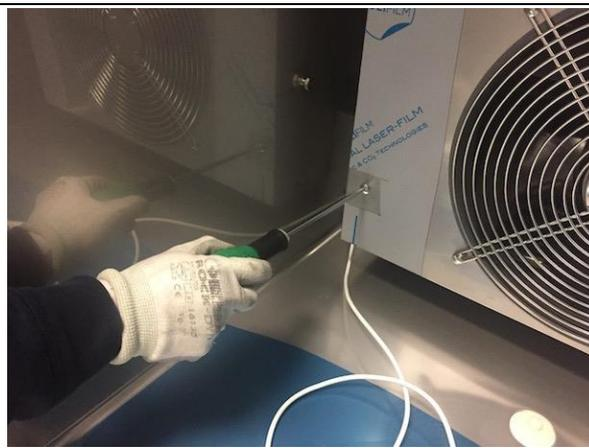
3. Loosen the evaporator support bracket screws
