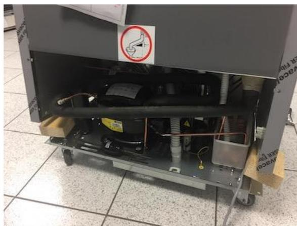
3. Move the discharge pipes to easily access the condenser.
