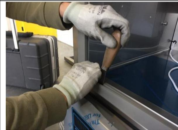
4. Take the lid with both hands and pull it towards you to remove it completely. Proceed in the same way for the other sides; in case of frame resistance replacement, go to the next step, otherwise jump directly to step [19](#).
