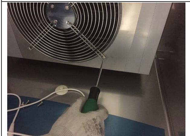
6. Cut the clamps that secure the power supply cable of the fan.
