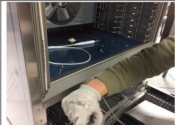
**20.** Proceed in the same way for the other sides until the lid/frame close properly and correct coupling on all corners.
