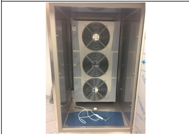
2. Open the evaporator conveyor by loosening its fixing screws.
