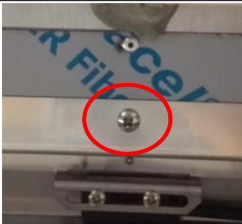
8. Remove the control panel by pushing it downwards and pulling it towards you.
