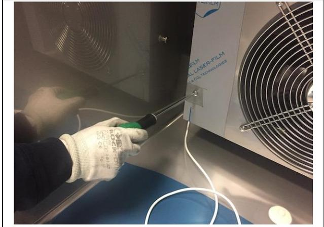
3. Loosen the evaporator support bracket screws
