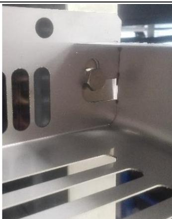
6. Remove the sealing grill of the filter cloth, arching it so that it comes out from its seat.
