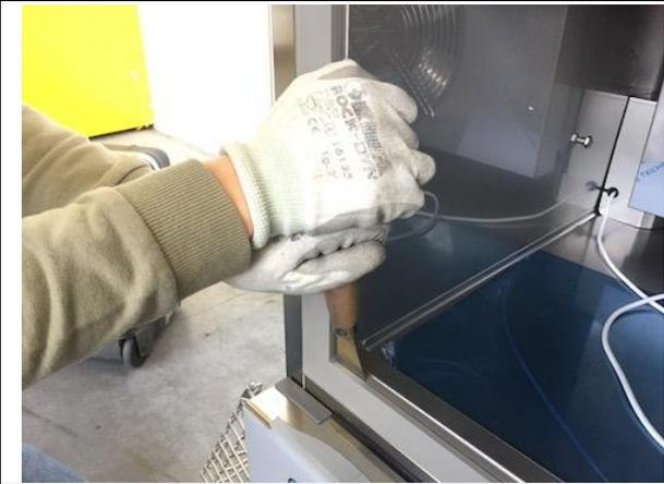
2. Using the spatula, force by tilting it towards the inside of the chamber and tapping it on the handle.
