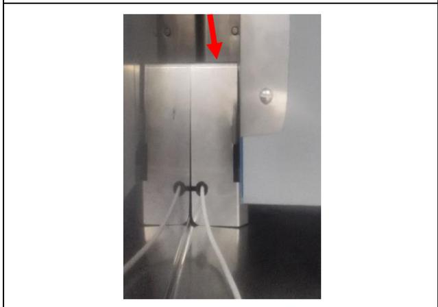
5. Cut the clamps that secure the probe cable.
