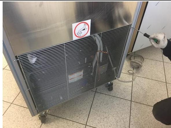
11. Cut the clamps that secure the fan power supply cable.
