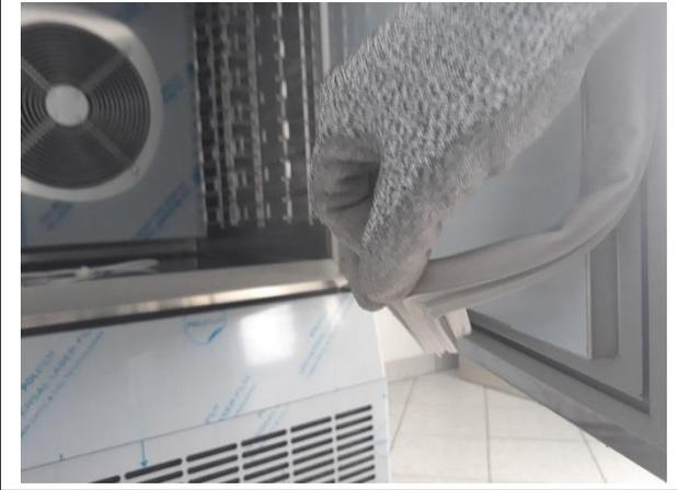
2. Position the new gasket by inserting it starting from the 4 corners and then pressing it along the respective sides.
