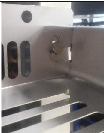
6. Loosen the hinge screws using the 8mm socket wrench.
