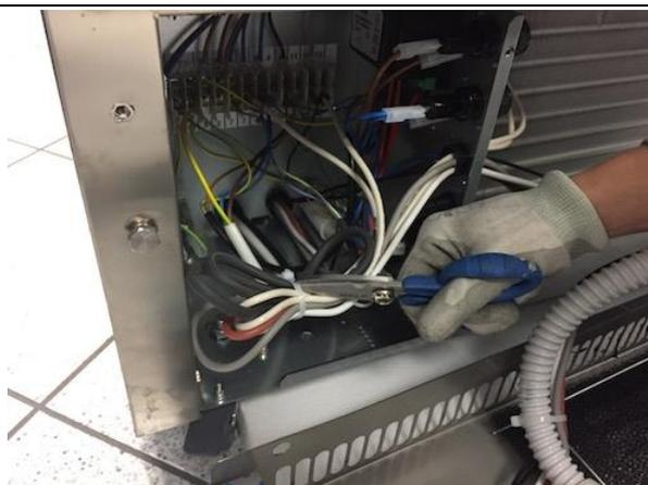
12. Remove the resistance from the frame and disconnect it from the terminal board terminals 7 and 10 [see wiring diagram, par.10].
