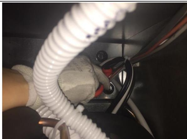
12. Pull the fan power supply cable downwards, taking care to do so as perpendicular as possible to the cell bottom.
