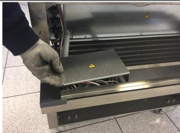
**14.** Disconnect the wires from card terminals 17 and 18 (if the probe is heated, disconnect the two additional ones also) [see wiring diagram, par. [10](#)].
