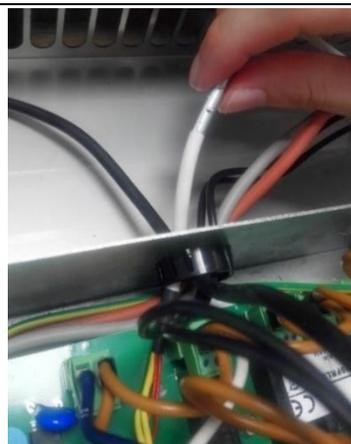
**19.** Connect the new probe to its terminal.
