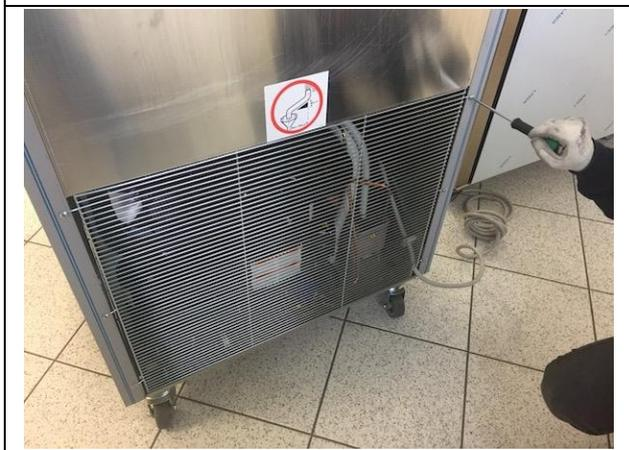
6. Cut the clamps that secure the probe cable.
