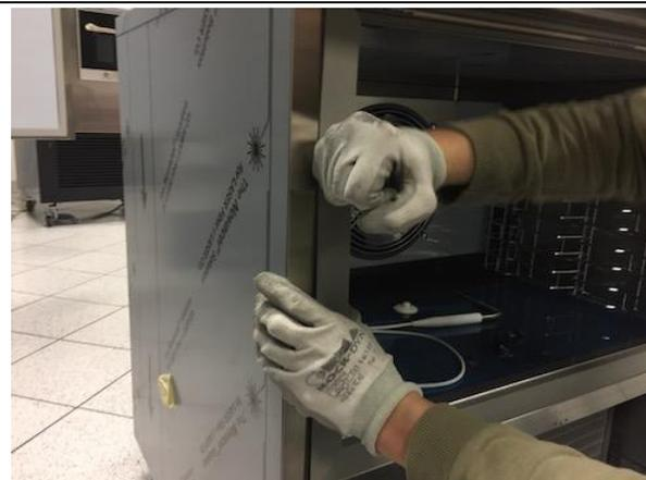
**21.** Seal all junction corners of the lids with sheet metal silicone.
