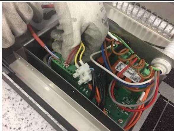
**15.** Remove any clamps and carefully pull the probe out.
