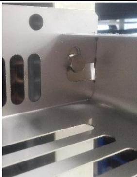
6. Loosen the hinge screws using the 8mm socket wrench.
