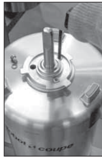
5) Remove bolts and washers
