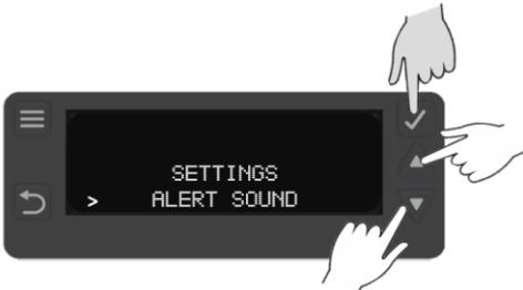
Press Select Button (2) to enter the ALERT SOUND option Press UP Button (4) & DOWN Button (5) to select value. Confirm your selection by pressing Select Button (2). Default is set to OFF.
