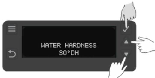
**STEP 6:** This Step is for the warewasher with External Water Softener Only. Set external Water treatment capacity in litres setting by using Up & Down buttons (5 & 6). Confirm the selection by pressing Select button (3). Refer supplier data for the external water softener device.
