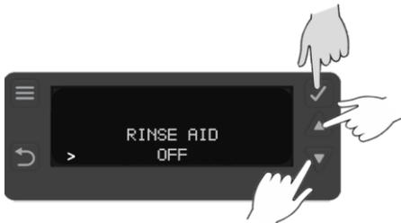
By pressing UP Button (4) & DOWN Button (5), you can set the chemical refill reminder notification ON. Press Select Button (2) to confirm the selection. Default is set to OFF.
