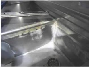
When limescale is found, it must be removed with commercial de-scaling chemicals, used with care in accordance with the instructions on the product.
