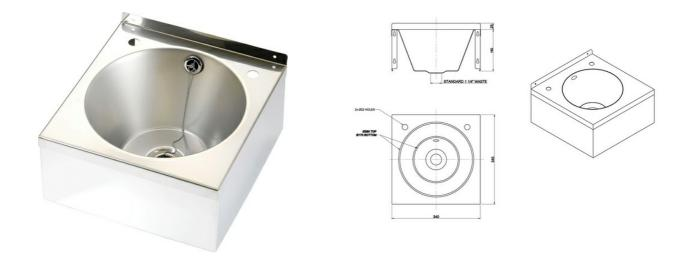
Washbasin top manufactured from 0.9mm thick, grade 1.4301 (304) stainless steel - high polish finish. The apron support is made from 0.9mm (430) material - high polish finish. Prepared for 32mm waste outlet overflow. Supplied with two tapholes in the rear ledge. Wall mounting by using the fixing holes provided in both the rear upstand and the rear apron fixing brackets. Screws and plugs are not supplied.
