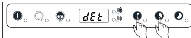
Fig.6 Detergent dispenser Manual Activation
