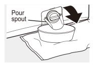
**4.** Turn the pump filter counterclockwise and remove the filter. Open slowly to allow the water to drain.
