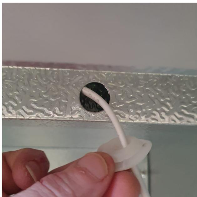
4. Pull out rubber ring from the top right hand side of bottle cooler interior.
