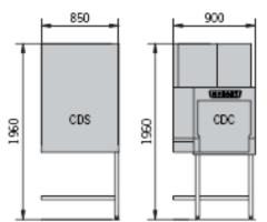
**CDS** straight dryer section adds 850mm to length of below machine & replaces 300mm exit "hood" as shown.
