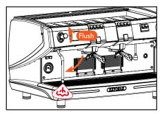
I. Aim the SmartSteam wand down towards the drip tray and tip the handle up to flush the steamer and eject any condensed water inside the system. If you have used your "SmarSteam" system after a long period of inactivity it's recommended to do a long flushing (6 to 10s) before frothing.
