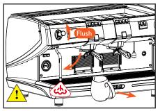
3. When the steaming is finished, remove the milk pitcher and wipe down the outside of the SmartSteam with a damp cloth to keep it always clean. Afterward, aim the SmartSteam wand down towards the drip tray and tip the handle up (for at least 3 seconds) to flush the steamer and eject any milk that may be in the steam tip
