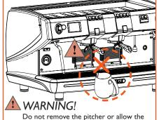
Do not remove the pitcher or allow the steam wand to extend out of the milk while steaming, it may cause serious burns and injuries.
