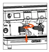
Unlock and remove the portafilter from the group head.
