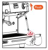
Place the steam wand over the drip tray and open the steam knob/handle for a few seconds to allow condensed water to be ejected. Close the steam knob/handle when only steam is coming out.
