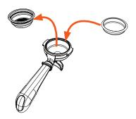
I. Remove the filter basket and place the blind filter in the portafilter.
