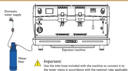
Connecting the machine to the domestic water supply must be performed by a qualified person.
