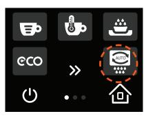
Enter the User Programming and select the Auto Cleaning cycle on the touchscreen. Automatic cleaning will start and lasts about one minute.
