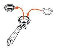
I. Remove the filter basket and place the blind filter in the portafilter.
