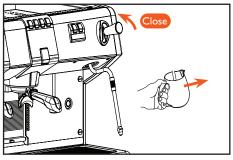
3. Once the milk reaches the desired temperature, close the knob/handle and wait for the steaming to stop, then remove the pitcher.
