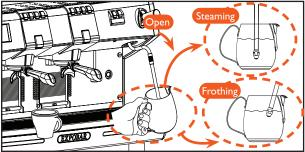
2. Immerse the steam wand into the milk, making sure the wand tip is submerged. Open the steam knob/handle again to begin steaming or frothing the milk. Always keep the tip of the steam wand submerged in the milk while steaming!
