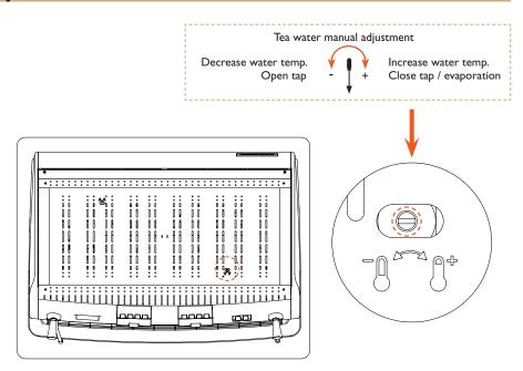
The Tea Water temperature can be adjusted manually using a flat blade screwdriver inserted into the temperature adjustment screw slot on the top of the machine as shown above.
