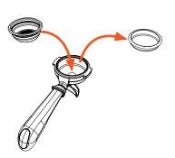
3. After rinsing, remove the blind filter and store it in a safe place for the next usage. Reinstall the filter basket in the portafilter.
