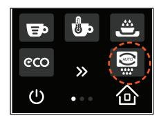
Enter the User Programming and select the Auto Cleaning cycle on the touchscreen. Rinsing will start and lasts about one minute.
