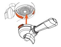
Align the portafilter's two flanges with the two slots in the group housing.
