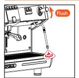
4. After steaming/frothing is finished, position the steam wand over the drip tray and open the steam knob/handle again for a few seconds to purge any milk remaining in the wand. Then wipe down the outside of the steam wand with a damp cloth to prevent nozzle blockage and to keep it clean.
