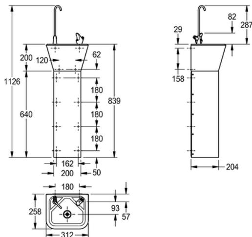
Drinking water fountains are manufactured from grade austenitic stainless steel, material thickness 1.2mm, supplied complete with 19mm waste and water bubbler. The wall mounted model is simply fixed to the wall using a joggle strip and integral mounting brackets. The pedestal version is fixed in the same way as the wall mounted version but incorporates extra fixing points within the pedestal support. No screws or wall plugs supplied.
