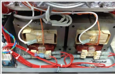
2000W e2s variant: two high voltage transformers side by side.
