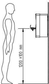
To comply with recommendations from the Health and Safety Executive it is important that due consideration be given to safe operation of the controls of the boiler. The boiler should therefore be mounted in such a manner that the operator can stand directly facing the machine with the controls at a recommended height from the floor to the draw-off tap handle of 1200mm +/- 100mm. Consideration should also be given to the servicing requirements of the machine.
