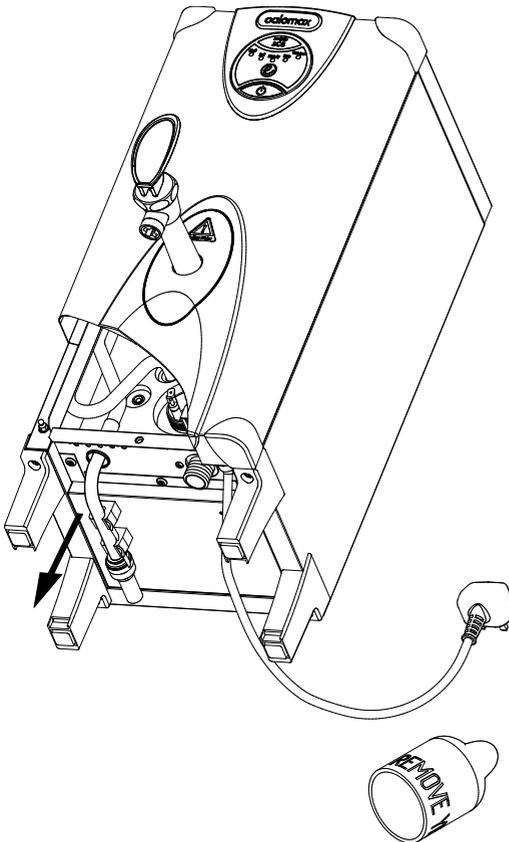
If the boiler is required to drip or overflow into the drip tray, the configuration of pipework may be altered as follows: Remove the machine front panel and unclip the pipework elbow. Carefully pull the elbow in the direction of the arrow, out of the silicone connecting tube on the end of the main water pipe. The silicone connecting tube will now direct water into the drip tray.
