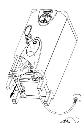
If the boiler is required to drip or overflow into the drip tray, the configuration of pipework may be altered as follows: Remove the machine front panel and unclip the pipework elbow. Carefully pull the elbow in the direction of the arrow, out of the silicone connecting tube on the end of the main water pipe. The silicone connecting tube will now direct water into the drip tray.
