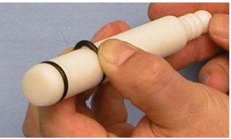
Figure 3-4 Removing O-Ring
