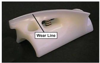
Figure 3-3 Auger Flight Wear
