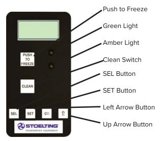
Figure 3-2 IntelliTec<sup>™</sup> Control
