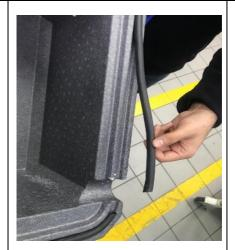
2) O-ring must be placed in its slot.
