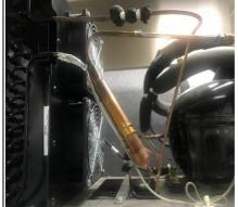
11) When the positioning is done the dryer mustn't touch with any surface.
