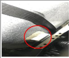
10) Vacuum Breaker must be sealed by putty on Freezer Cabinets, it must be also checked by service technicians!
