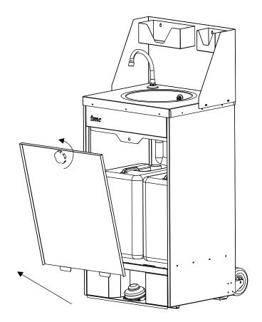
Once the front panel has been removed, lift out the suction hose from the clean water container and remove the water container. Note the water container can hold a maximum of 20 litres. Ensure when refitting the water container that the suction hose has been placed at the bottom container.
