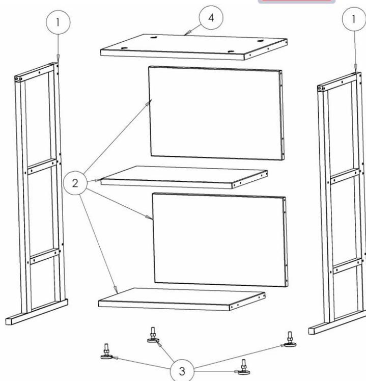
1. Screw M12 locking nut (item 5.7) onto adjustable foot (item 3), 4 off, then screw foot fully into base of end assembly frames. Do not tighten locking nuts.
