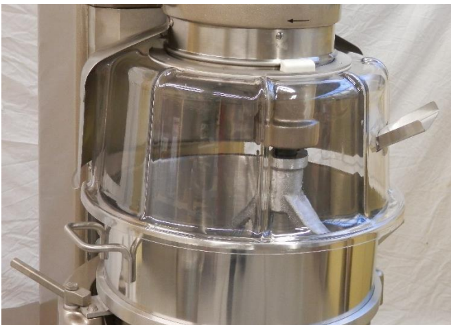
1. Solid dust guard closed with ingredient chute fitted.
