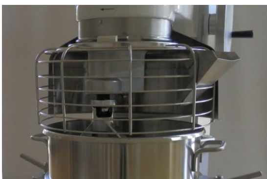
1. Wire cage guard closed with ingredient chute fitted.
