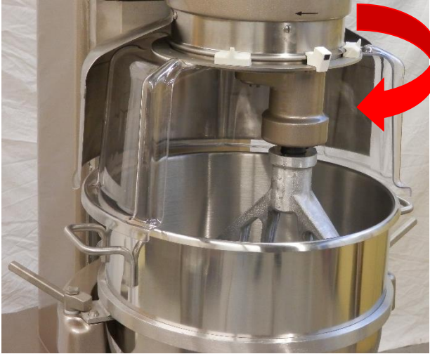
3. Open the guard rotating clockwise/to the left.
