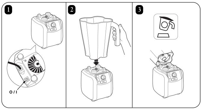
The location of the main power switch will be either on the front of the unit or on the bottom of the unit as indicated above.
