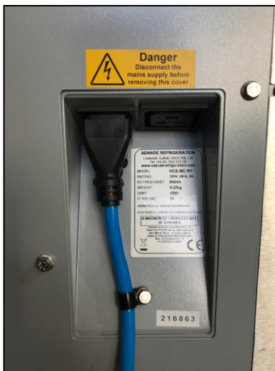
Figure 3: Mains connection point
