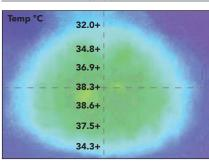
Thermal image depicting temperatures in degrees Celsius when HQ900E lamp positioned 500 mm above surface.
