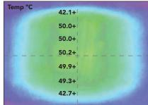
Thermal image depicting temperatures in degrees Celsius when HE900 lamp positioned 500 mm above surface.
