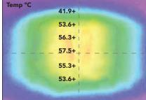
Thermal image depicting temperatures in degrees Celsius when HE900 lamp positioned 400 mm above surface.
