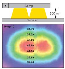
Thermal image depicting temperatures in degrees Celsius when HQ900E lamp positioned 300 mm above surface.
