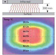
Thermal image depicting temperatures in degrees Celsius when HE900 lamp positioned 300 mm above surface.
