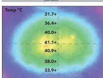
Thermal image depicting temperatures in degrees Celsius when HQ900E lamp positioned 400 mm above surface.
