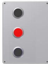
Solid Red WARNING! – Bin Not Present Machine Stopped
