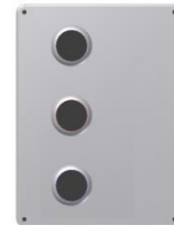
No Lights Machine Stopped No Warnings
