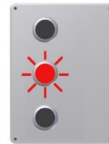
Flashing Red WARNING! – Bin Full Machine Stopped
