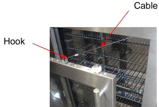
Un-hook the cable from the hook in the top of the door, the door can now be fully removed from the unit
