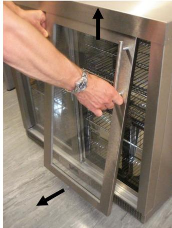
To remove the door lift the door upwards and swing the bottom out from the bottom roller guide
