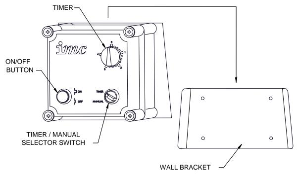
Note: Control boxes for three phase machines have separate on and off buttons.
