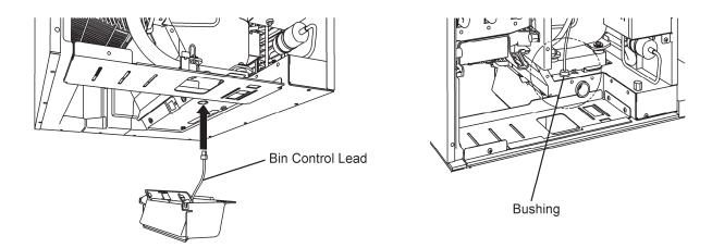
7) While pulling up the bin control lead, hook the bin control on the right side interior wall. Then push the bin control up against the bottom of the unit, and slide to the back until it snaps in place. Make sure the slotted holes at the right side of the bin control are securely placed on the collars at the bottom of the unit.
