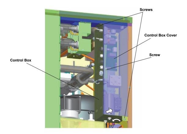
Note: After replacing the components inside the control box, connect and tie the wires properly in their correct position. Especially make sure that the harness does not press the push buttons on the control board.
