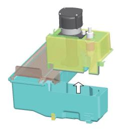
3) Flip over the pump motor bracket assembly, then twist off the float switch and pull out towards you.
