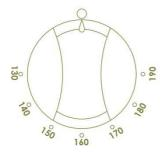
The fryers are controlled by a thermostat which offers settings between 130 and 190°C.
