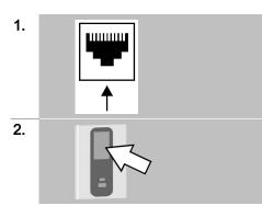
Use a network cable to connect the network socket on the combi oven to the network socket which the customer has pre-installed and given clearance for use.
