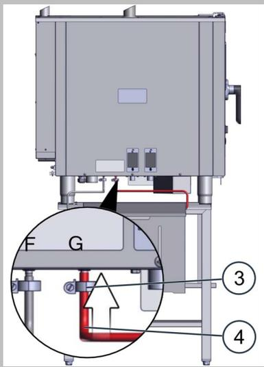
Plug the red extractor tube (4) for the ConvoClean forte or ConvoClean new cleaning agent onto the connector nipple of the front tube fitting (G) and secure the tube in place with the wire clip (3) (see label for cleaning-agent connection on the left-hand side of the appliance).
