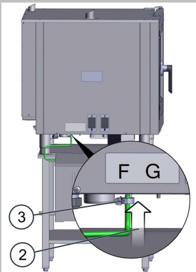
2. Plug the green extractor tube (2) for the ConvoCare rinse aid onto the connector nipple of the rear tube fitting (F) and secure the tube in place with the wire clip (3) (see label for rinse-aid connection on the left-hand side of the appliance).
