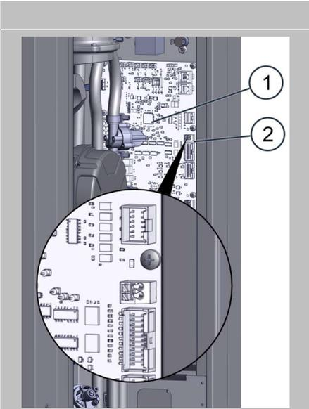
Remove the side panel from the combi oven in order to access terminal block X33 (2) on the system interface board (SIB) (1) in the area behind the operating panel.
