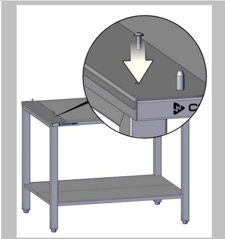
Screw the two adapter plates to the stand using two socket screws each.
