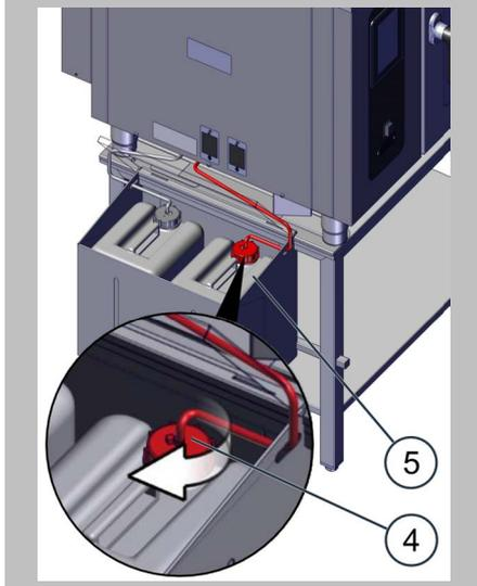
Insert the suction nozzle on the red extractor tube (4) into the cleaning-agent canister (5). There must be no kinks in the tube and the vent hole in the canister must be open and unblocked.
