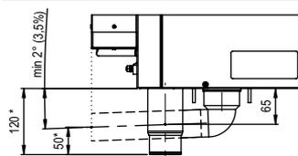
\* Distance depends on how far the appliance feet are extended (max. +25 mm)
