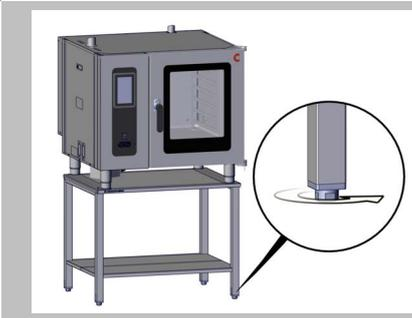
Ensure the stand is horizontal by adjusting the height of the feet.
