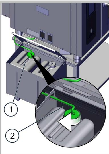
3. Insert the suction nozzle on the green extractor tube (2) into the rinse aid canister (1). There must be no kinks in the tube and the vent hole in the canister must be open and unblocked.
