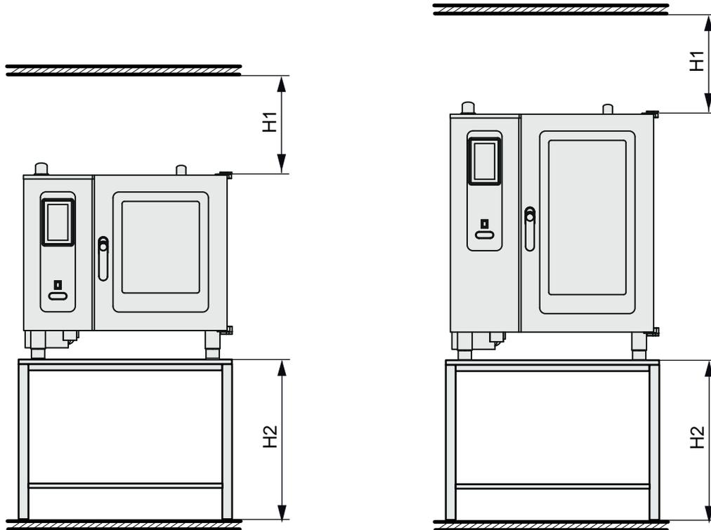
The service engineer who is responsible for setting up the appliance must take into account the nature of the ceiling and any adjacent systems that may be used (air ventilation system, vapour extractor hood etc.) when designing the particular clearance needed between the top of the appliance and the ceiling. In this context, the vertical distance H1 must be understood as a guide value for the minimum vertical clearance.
