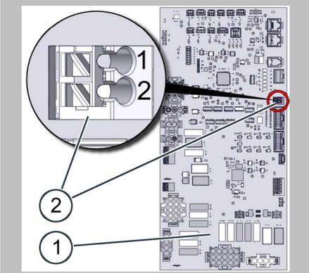
Connect the connecting cable to the combi oven in accordance with the PIN assignment shown below.
