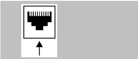
Use a network cable to connect the network socket on the combi oven to the network socket which the customer has pre-installed and given clearance for use.
