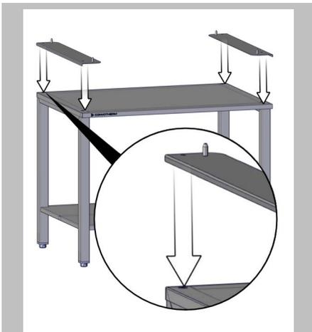
Place the two adapter plates on the stand, with the locating pins pointing upwards.
