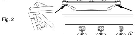
The Pan Supports can be cleaned with a mild detergent and hot water solution using a soft bristled brush. Rinse and dry thoroughly with a dry cloth.
