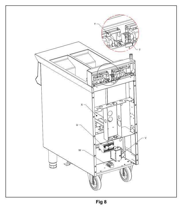
T Element microswitch U Contactor block X Wiring cover Y Swivel cover clip
