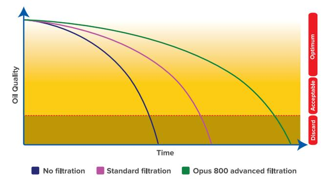
Highly efficient filtration system extends oil life by up to 75%
