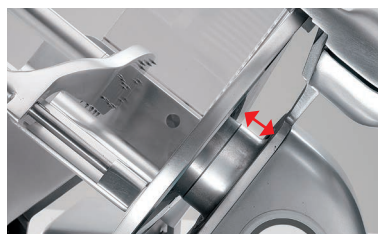
Increased gap between blade and machine body
