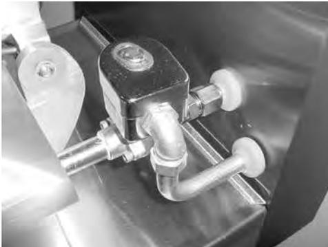
1. Remove Tru-Arc retaining clip on top of the coil housing.
