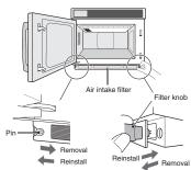
The timing to clean the air intake filter will be announced by the "CLEAN CAUTION" indicator and sound. After maintenance, press the STOP/CLEAR pad for 2 seconds to turn off the indicator.
