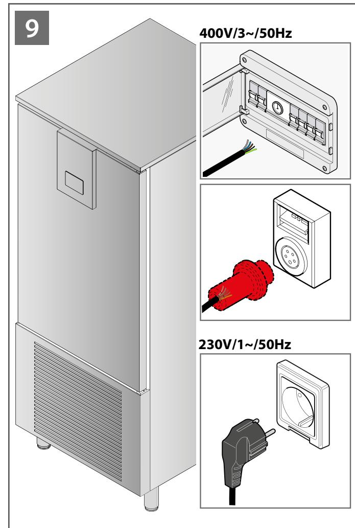
those indicated in the device serial number plate. A rated voltage variation of +/-10% is accepted.
