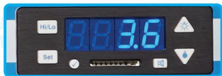
The simple to use four button controller displays the internal temperature of the fridge, but it also shows minimum and maximum temperatures which can be displayed at the touch of a button. It also alarms if the internal temperature drops below 0°C or rises above 5°C. The Breast Milk fridge is also fitted with a door open alarm and, if batteries are fitted, a mains failure alarm.
