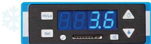
The simple to use four button controller displays the internal temperature of the fridge, but it also shows minimum and maximum temperatures which can be displayed at the touch of a button. It also alarms if the internal temperature drops below 0°C or rises above 5°C. The Breast Milk fridge is also fitted with a door open alarm and, if batteries are fitted, a mains failure alarm.
