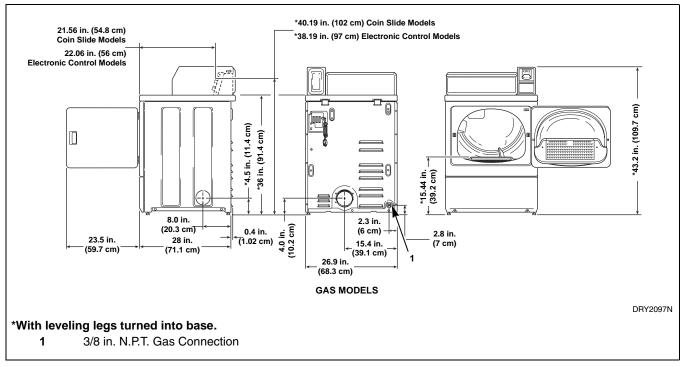
NOTE: Side, rear and bottom exhaust openings are 4 inch (10.2 cm) ducting. Gas models cannot be vented out left side of cabinet because of burner housing.
