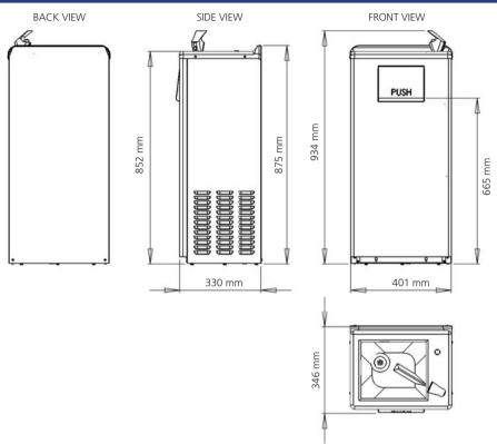
Can be used free standing or wall tight to avoid unsightly connections. Exclusive Projector Design: 2-stream mound-building projector and automatic stream regulator. Plumbing Connections: enter directly into cabinet. Waste 24 mm (1") IPS.
