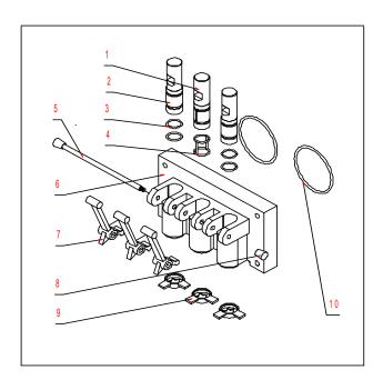
**ITEM** Part Number QTY. Description 1 1 T29206007 Middle Dispensing Valve 2 Side Dispensing Valve T29206004 2 3 T29206006 4 O-ring 4 1 T29206002 O-O ring 1 5 Dispensing Handle Retention T29206005 1 6 T29206001 Dispensing door 7 T29206008 3 **Dispensing Handle** 8 2 T29206009 Screw cap 9 3 T29206003 Design Cap 10 T29020601 2 Seal of Dispensing Door
