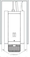
\* Required for ventilation if the machine is installed in an enclosed cabinet
