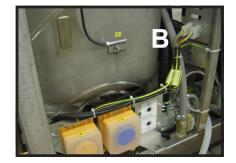
Connect the plug (B) of the wire harness with the dosage pump (max. 100 VA).
