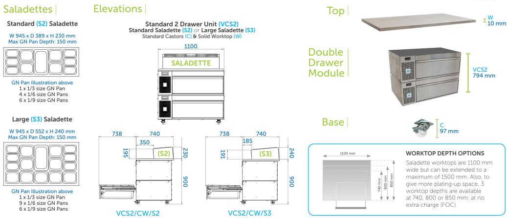
OPTIONS (Note: due to rounding differences, the dimensions for Drawer Module + Top + Base may vary by 1 mm compared to the dimensions shown below)
