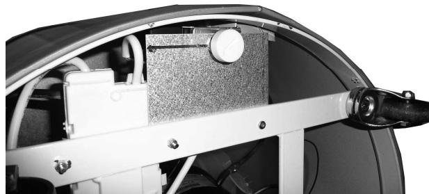
The thermostat is placed under the cabinet. The thermostat can be positioned from app. 0 to 10 °C. A positioning in app. the middle of the scale will in most cases be ideal. Turn the thermostat button clockwise if the temperature is too high or anti-clockwise if the temperature is too low.
